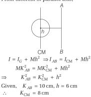
24 The theorem of parallel axis for moment of inertia.
