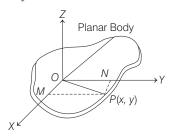
If  $I_x$  and  $I_y$  be moment of inertia of the body about two perpendicular axes in its own plane and  $I_z$  be the moment of inertia about an axis passing through point O and perpendicular to the plane of lamina, then
